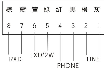
Figure 2-4 RJ-45 Connector
